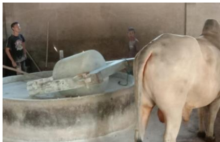
Figure 1 Cylinder, a place to mix tapioca flour and cassava flour with the help of cow power (source: 2022 Field Observations)
