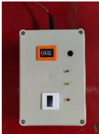
Figure 4. Results of Brake Fading Early Warning Device Design
