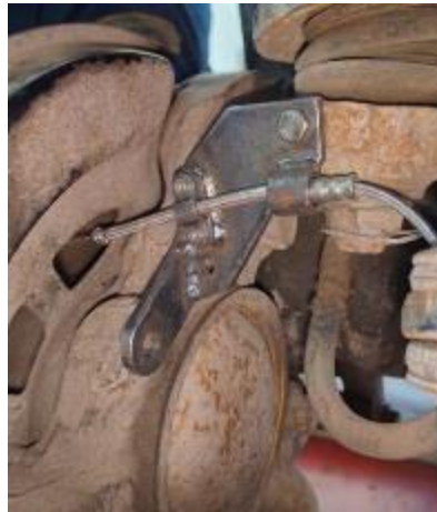
Figure 3. Thermocouple Sensor Installation on the Disc Brake
