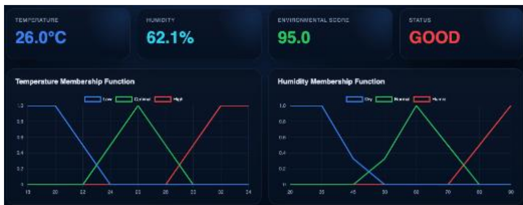
Figure 5. Temperature and humidity membership functions and the corresponding environmental assessment result
