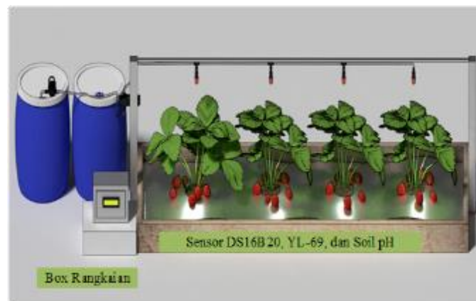
Gambar 5. Desain alat monitoring tanaman stroberi
