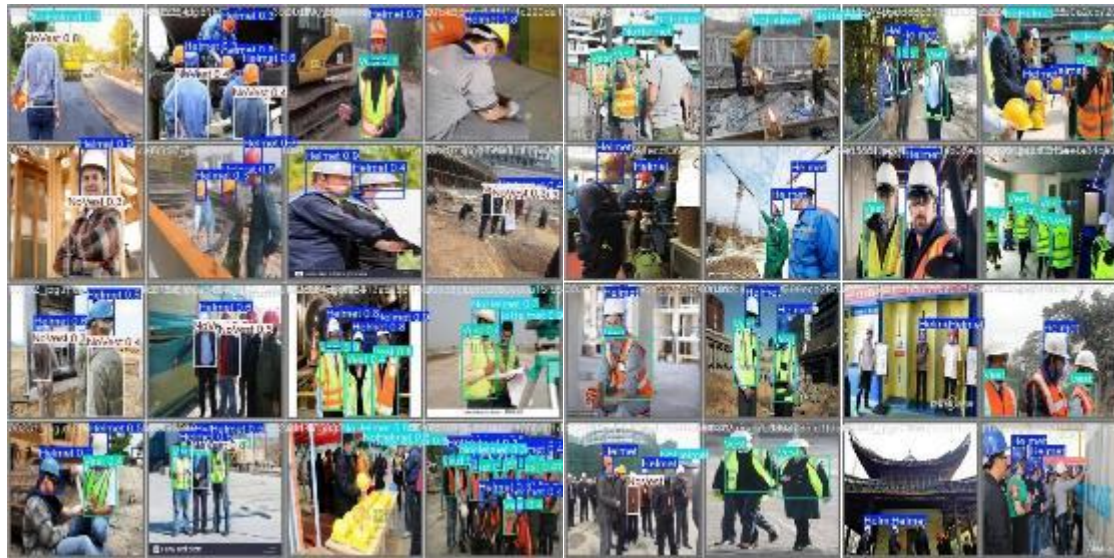
Figure 12. PPE detection in technicians/operators by Model
