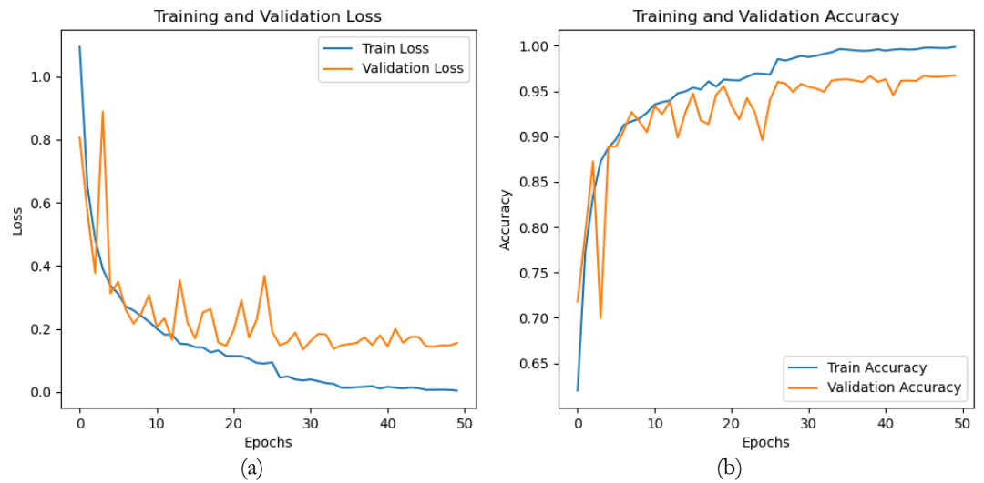
Figure 2. Training and validation loss (a) and accuracy (b) curves of EDANet over 50 epochs.
