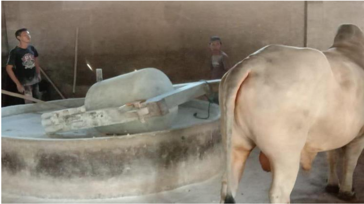
Image 1 Cylinder, a place to mix tapioca flour and cassava flour with the help of cow power
